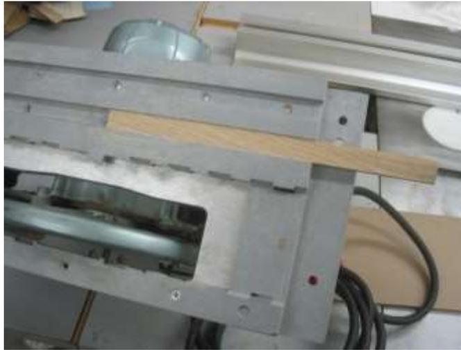
Started by ripping a piece of 3/16" thick oak for a snug sliding fit in the base groove.
