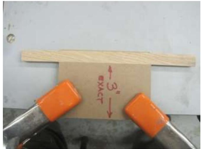
Ripped a second piece of  $\frac{1}{4}$ " MDF to 3-3/4" wide, clamped the 3" piece to it with the edges aligned as shown and stuck the oak strip to it using double-sided tape – this locates the edge of the fixture at 3" from the edge of the groove.
