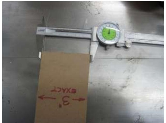
Ripped a piece of 1/4" MDF to 3" wide – the required distance from the base groove to the inside face of the saw blade. This part will be used to establish the 3" dimension from the edge of the fixture to the edge of the track groove in the bottom of the EZ Saw Base.
